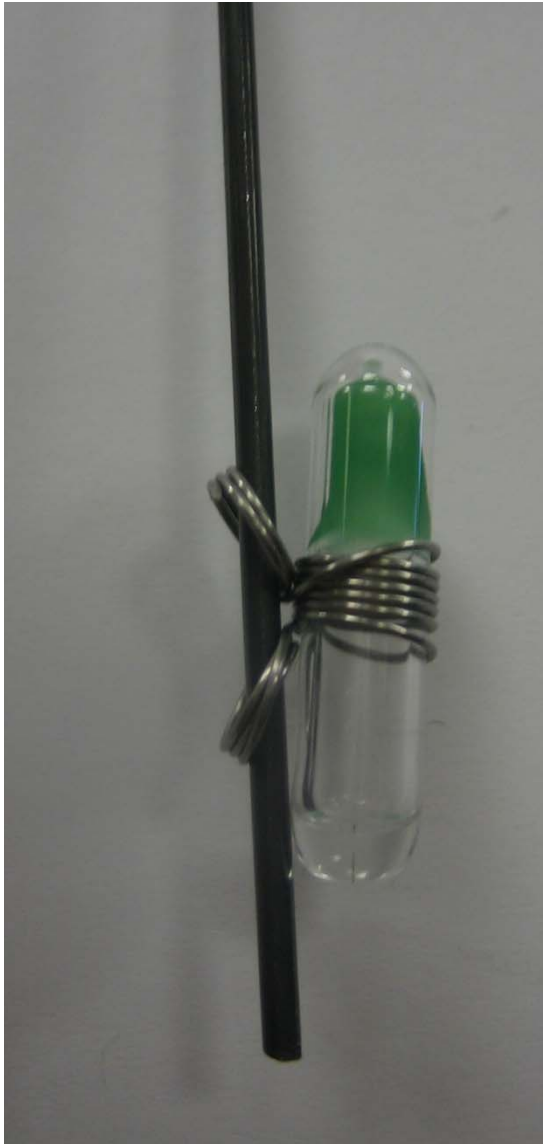
Figure 2: The Water Pasteurization Indicator available from Solar Solutions (glass tube only). The rod and spring arrangement turns the simple glass tube indicator into a general purpose indicator that can be used in many different shapes of water vessels.
