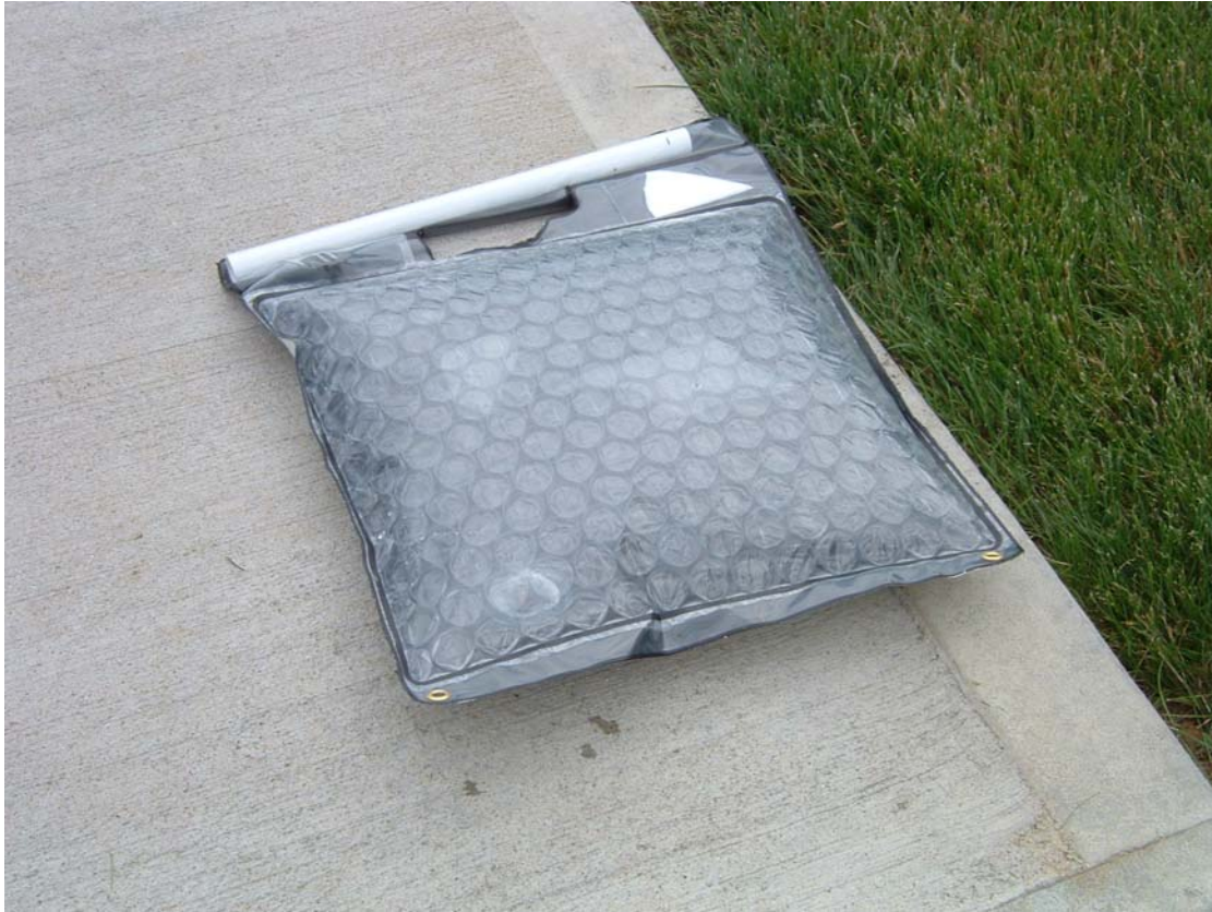
Figure 8: The AquaPak. The bubble wrap in the top insulating layer is visible. Here, the AquaPak lies directly on the ground, where the only bottom insulation is the ¼ inch (6mm) foam layer built into the bottom of the AquaPak. Slightly better performance can be achieved by laying the AquaPak on some insulating material such as grass or leaves.
