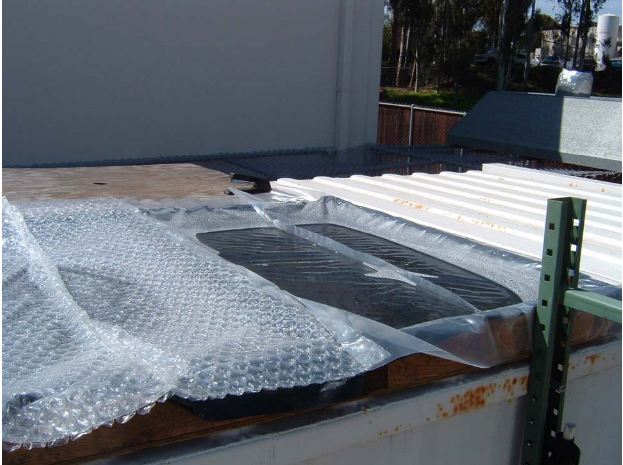
Figure 12: Photograph showing two versions of the solar puddle built on a platform. The version on the right is the standard version, normally with 4 layers of plastic but the top layer has been removed. The version on the left has the top two layers of plastic replaced by bubble wrap. Both versions perform about the same.
