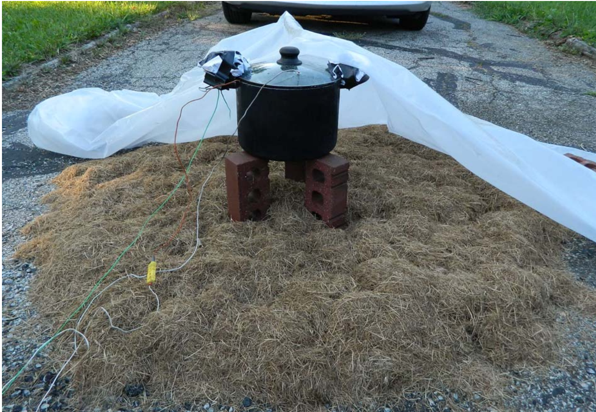
Figure 4: A small pot-based water heater. The pot holds 6.8 liters of water. The cover sheet is partially folded back for visibility.
