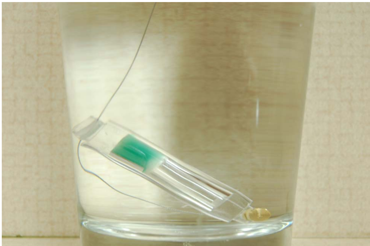
Figure 1: The Water Pasteurization Indicator (WAPI, or Indicator) available from Solar Cookers Int'l.
