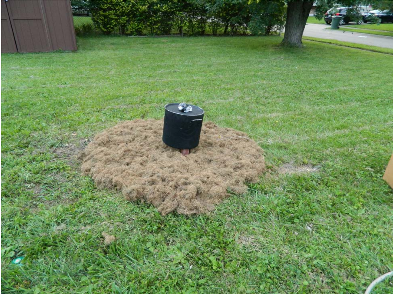
Figure 5: A large pot-based heater, shown without the cover. The pot holds about 29 liters of water.
