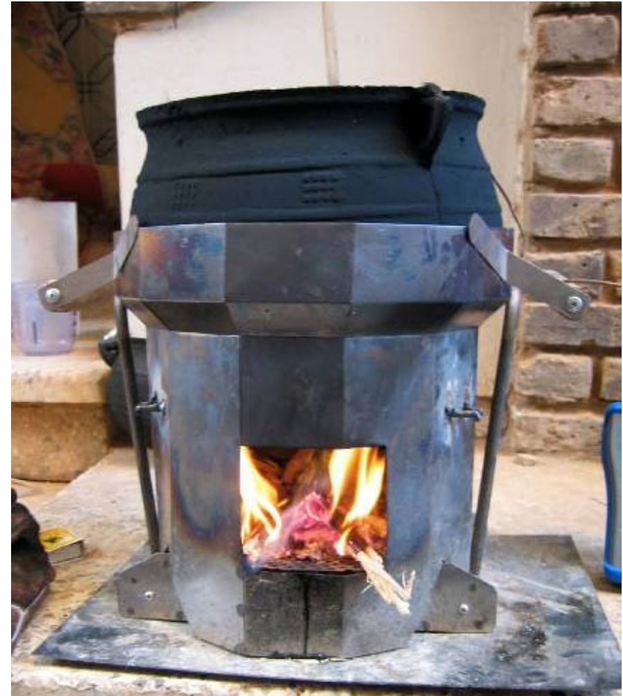
First Field Tested Prototype, 2007 (Berkeley-Darfur Stove version 5)
