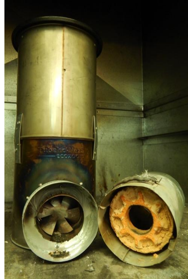
Mixing by fan and orifice. Secondary air is introduced downstream of the orifice.
