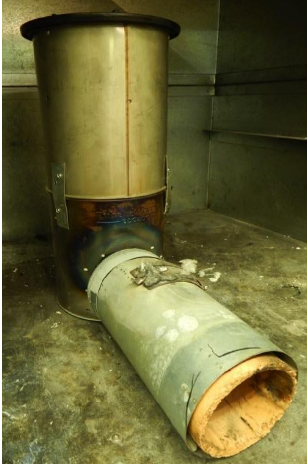
Rocket stove with horizontal "TLUD" combustion chamber
